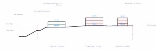
INDICATIVE SECTION BB - LEVELS OF PROPOSED UNITS IN THE CONTEXT OF THE RIVER BANK
