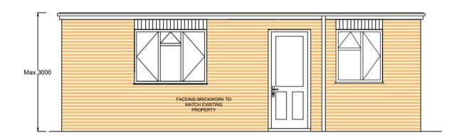
FRONT ELEVATION PROPOSED- SCALE 1:50
