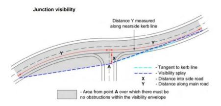
Figure 3: Typical Visibility Splay diagram
