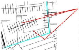
The dotted lines here show that the ground was not a uniform level across the entire site. This is taken from the owners original application and shows there is variation. Which is the reason sheet piles have been used to raise it.
