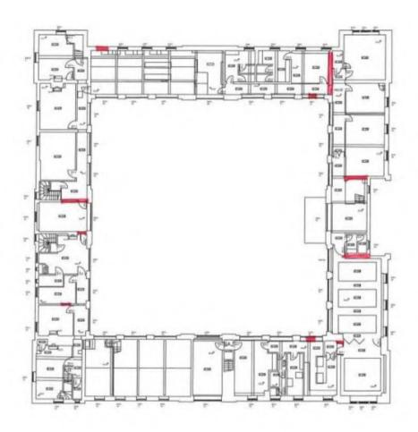
Revised extent with reduced removal of original fabric in apartment wing
