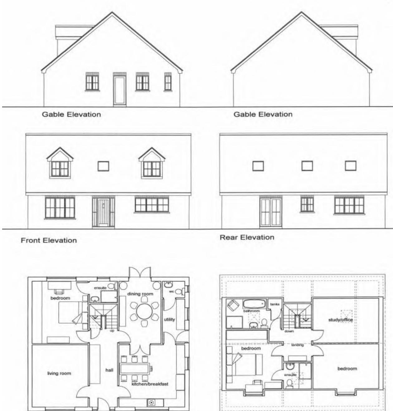
Proposed elevations and floor plans
