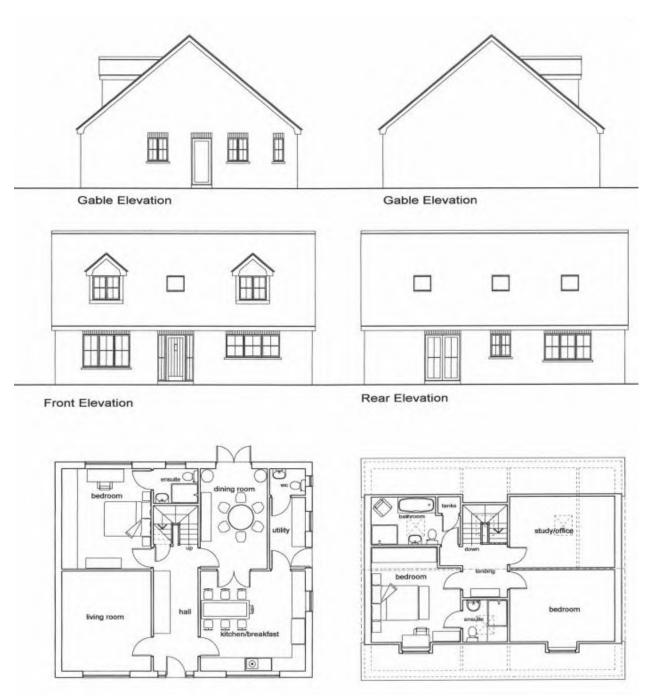
Proposed elevations and floor plans
