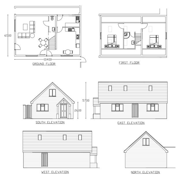
The conversion involves the insertion of rooflights in the pitched roof and a new window in the northern elevation at first floor level.
