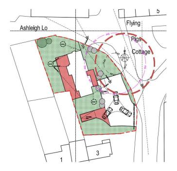
The only aspect of the works that would be within the root protection area is the proposed driveway. This is therefore proposed to be constructed with a cellular design to prevent ground compaction to the surface of the driveway by vehicles, thus protecting tree roots below ground. The cellular design is illustrated at Appendix E. This will be conditioned in the event of an approval.
