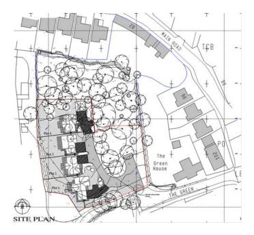
The illustrative layout shows the retention of the on-site pond and the retention of the large majority of the on-site trees. Those trees that are shown as being felled are primarily the fruit trees within the small orchard.
