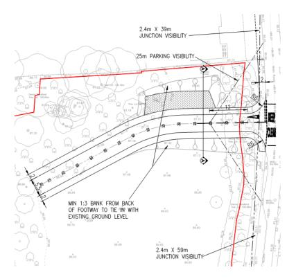
The area with the herringbone hatching is the area intended to be offered as car parking space for users on the village hall. It would have a useable width of approximately 20 metres and would therefore accommodate up to eight vehicles. The distance between the car parking and the hall itself would be approximately 32 metres.
