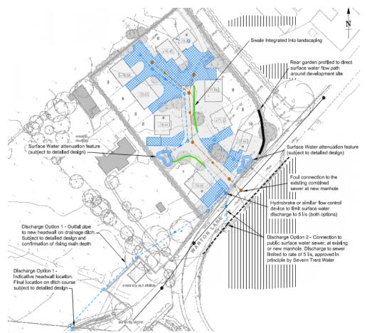
The applicant argues that, in terms of off-site impacts, the current greenfield runoff is likely to contribute to the known overland flooding issues on Warton Lane. The introduction of a formal drainage system on the site will ensure that flows from this site are controlled and managed. In addition, the proposed downstream outfall may provide a positive impact on the surface water flooding on Warton Lane.
