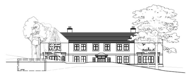
Proposed Front Elevation (in context of ground levels and showing sunken garage)
