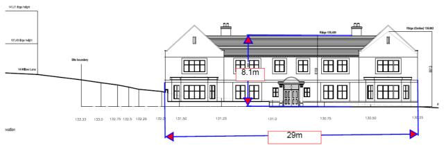
Proposed Front Elevation (showing comparative height to properties on Mill Lane)
