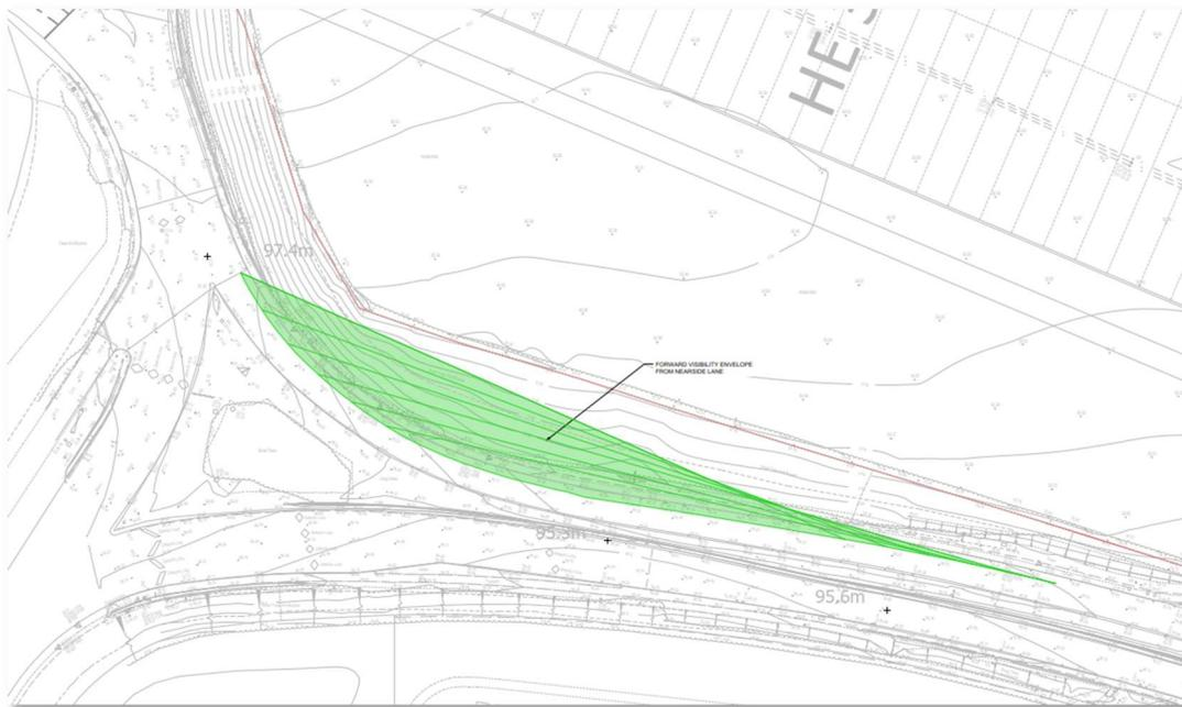
**Plate XII:** Extract from drawing produced by Dr Nick Bunn. Green shaded area shows extent of vegetation that needs to be reduced to approximately 0.26m above ground level in order to provide the necessary forward visibility.
