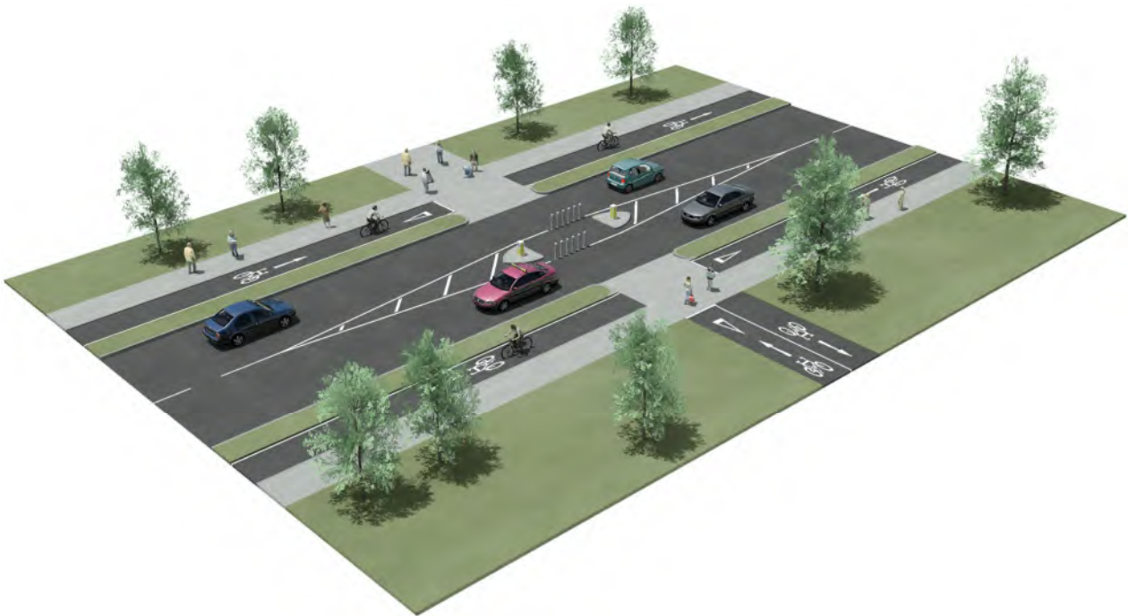
Example of controlled pedestrian and cycle crossing
