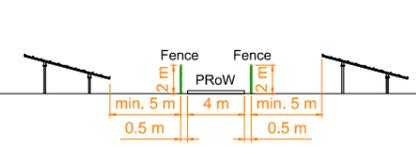
Typical Elevation for PV Array
