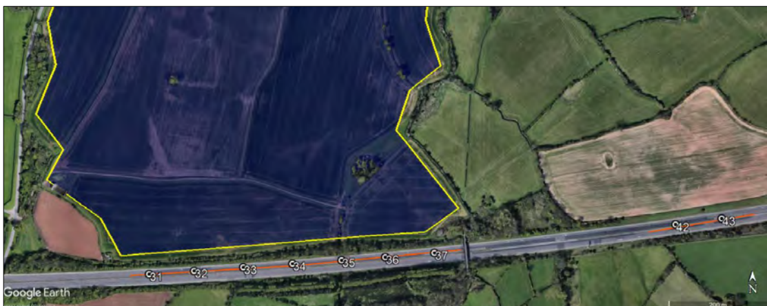
Figure 32 – Stretch of M6 where solar reflections are predicted to be geometrically possible and relevant screening
