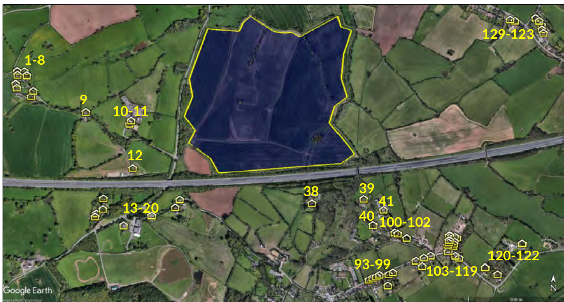
Figure 10 – Dwellings where solar reflections are geometrically possible
