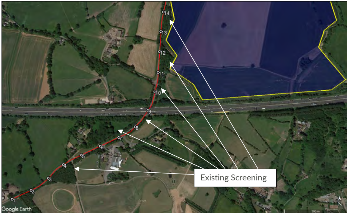
Figure 11- Stretch of B4102 where solar reflections are predicted to be geometrically possible and relevant screening
