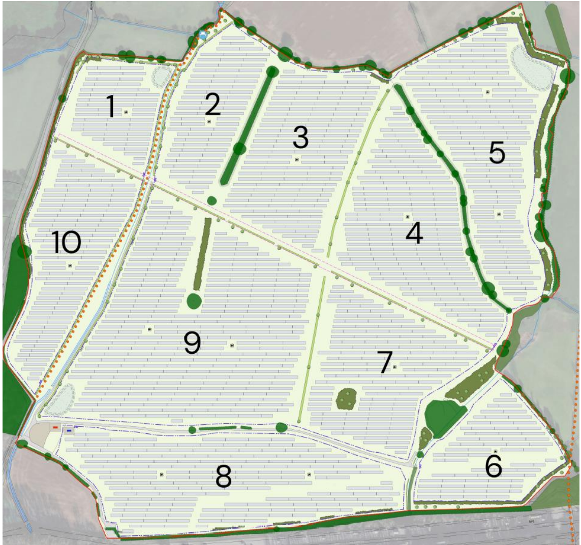
Plate 2: Extract from the proposed Landscape Strategy Plan detailing the location of the proposed solar arrays, associated infrastructure and landscaping (included within Appendix 8 of the evidence of Mr Cook; DRWG: P24-1827_008).
