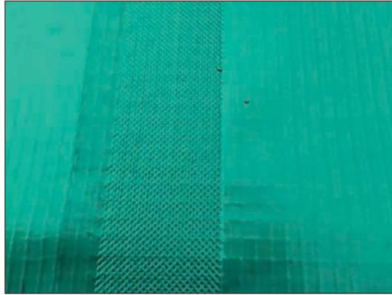
**Figure A4.62** Wedge weld on an LDPE aluminium gas membrane, where the installer used metal nip rollers. This destroyed the top layer and probably the bottom layer, leaving aluminium exposed between the weaves. This failed dielectric testing along all joints (courtesy MEC Environmental Ltd)
